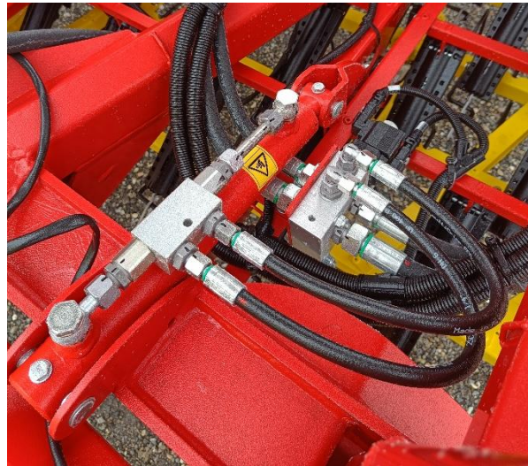
Figure 11: hydraulic cylinder and electromagnetic valve
