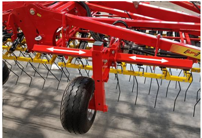
Figure 12: adjusting the feeler wheel track
