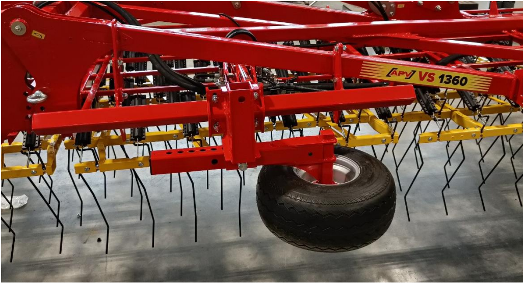
Figure 7: feeler wheels on the side frames in transport position
